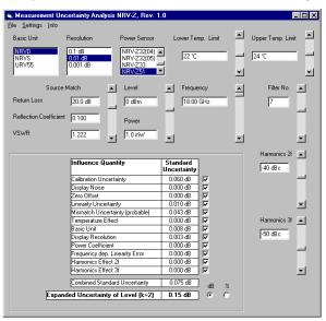
Basic unit, resolution and sensor type are selected by clicking on the appropriate list. To select a power sensor that is not visible in the first four lines of the list, use the scrollbar on the right.
